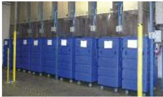
Sorting machine which is used to automatically sort linens before being washed.
