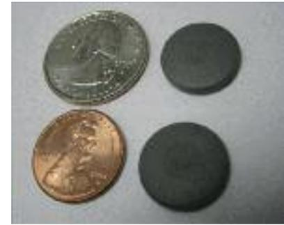
RFID chip compared to the size of a coin.
